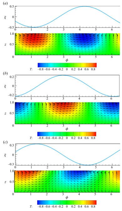
Figure 8. The perturbation flow field and surface deformation at Pr = 0.01, Ca = 0.001 and G = 100: (a) Bo = 0,  $\zeta = 0$ ; (b) Bo = 10,  $\zeta = 0.5$ ; and (c) Bo = 0,  $\zeta = 0.49$ . The perturbation phase is defined as  $\phi = \alpha x + \beta y$ .
