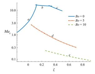
Figure 6. The variation of  $Ma_c$  with  $\zeta$  and Bo at Pr = 0.01. The curves correspond to streamwise waves of SWI (a, c, d and e) and the oblique wave of CI (b).
