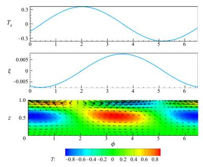
Figure 13. The perturbation flow field and surface deformation at Pr = 100,  $\zeta = 0.4$ , Bo = 5, Ca = 0.001 and G = 100. The preferred mode is the downstream streamwise wave. Here,  $T_s$  is the perturbation temperature on the surface.
