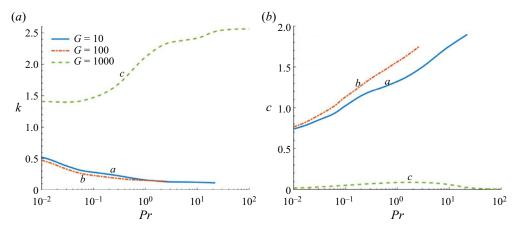
Figure 3. The (a) wavenumber and (b) wave speed of the modes in figure 2.
