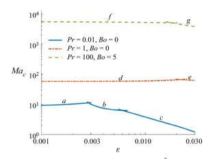
Figure 14. The variation of  $Ma_c$  with  $\varepsilon$  at  $\zeta = 0.49$ , Bo = 0 and  $\tilde{\beta} = 0.1$ . The curves correspond to downstream streamwise waves (a, b, c, d and f) and upstream oblique waves (e and g). SWI includes curves a, b, d and f, while CI includes curves c, e and g.
