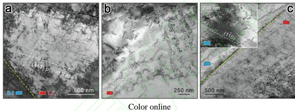
图 12 Al<sub>19</sub>Co<sub>20</sub>Fe<sub>20</sub>Ni<sub>41</sub> 共晶高熵合金两相组织的低温变形特点<sup>[100]</sup>**Fig.12** Deformation feature of dual-phases in Al<sub>19</sub>Co<sub>20</sub>Fe<sub>20</sub>Ni<sub>41</sub> eutectic high-entropy (EHEA) alloy at cryogenic environment<sup>[100]</sup>
