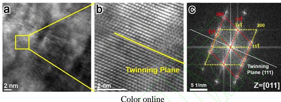
图 5  $\text{Al}_{3.6}\text{Co}_{27.3}\text{Cr}_{18.2}\text{Fe}_{18.2}\text{Ni}_{27.3}\text{Ti}_{5.4}$  高熵合金中  $L1_2$  析出相低温变形后的孪晶特征<sup>[68]</sup>**Fig.5** Nano-twins in  $L1_2$  precipitate in  $\text{Al}_{3.6}\text{Co}_{27.3}\text{Cr}_{18.2}\text{Fe}_{18.2}\text{Ni}_{27.3}\text{Ti}_{5.4}$  alloy after deformation at 77 K<sup>[68]</sup>
