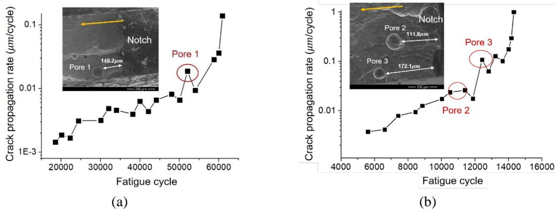
**Figure 2.** Fatigue small crack propagation rate curve and fracture morphology of SLM AlSi10Mg alloy at (a) room temperature; (b) 400°C
