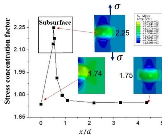
Figure 6. Maximum stress concentration factor around the pore and finite element analysis results
