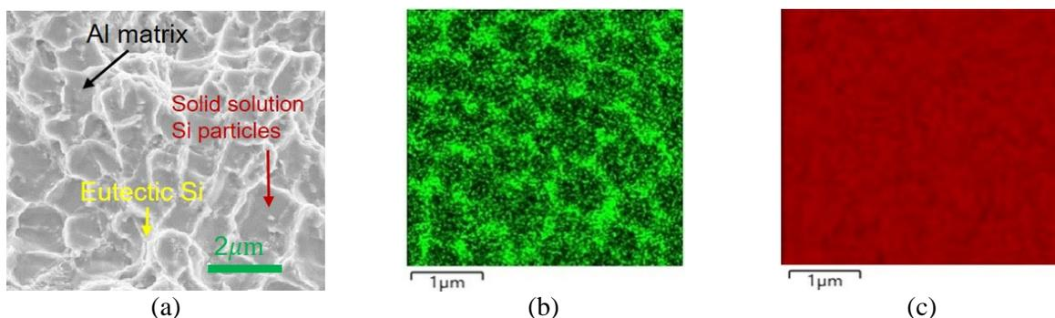
**Figure 4.** (a) Microstructure of SLM AlSi10Mg alloy; Composition distribution of (b) Si element; (c) Al element
