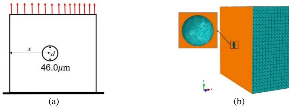
Figure 5. (a) Schematic diagram of representative volume unit; (b) Finite element model
