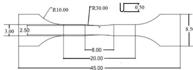
**Figure 1.** Geometry size of the SLM AlSi10Mg fatigue specimen (unit: mm)
