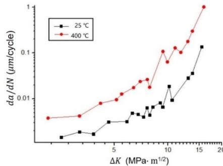
**Figure 3.** Relationship between stress intensity factor amplitude ( $\Delta K$ ) and crack growth rate ( $da/dN$ )
