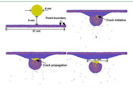
**Figure 7.** Deformation and failure mechanism from MD simulations of the Ni<sub>2</sub>Ta MG nanofilm with a thickness of 1 nm at impact velocity  $v_i = 3$  km s<sup>-1</sup>.
