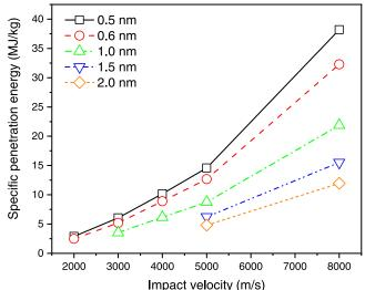
**Figure 5.** Specific penetration energy  $(E_p^*)$  of the Ni<sub>2</sub>Ta MG nanofilms with different thicknesses and impact velocities from MD simulations. For 1.5-nm-thick and 2.0-nm-thick films, the films are not fully penetrated at impact velocities lower than 5 km s<sup>-1</sup>.
