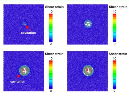
Figure 8. Deformation behavior and shear strain distribution of the Ni<sub>2</sub>Ta MG nanofilm with a thickness of 1 nm at the impact velocity  $v_i = 3 \text{ km s}^{-1}$ .
