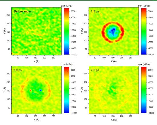
Figure 6. Stress wave propagation ( $\sigma_{xx}$ ) from MD simulations of the MG nanofilm with a thickness of 3 nm at impact velocity  $v_i = 4$  km s<sup>-1</sup>.
