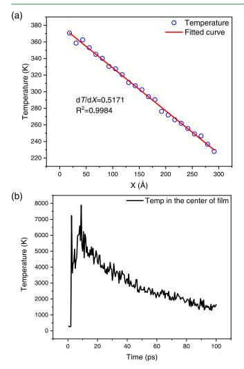
**Figure 9.** (a) Radial distribution of temperature of the Ni<sub>2</sub>Ta MG nanofilm from MD simulations. This was used to estimate the thermal conductivity *k* of the Ni<sub>2</sub>Ta MG nanofilm, leading to k = 9.7 w (m k)<sup>-1</sup>. (b) Temperature evolution at the center of the Ni<sub>2</sub>Ta MG nanofilm during impact from MD simulations.
