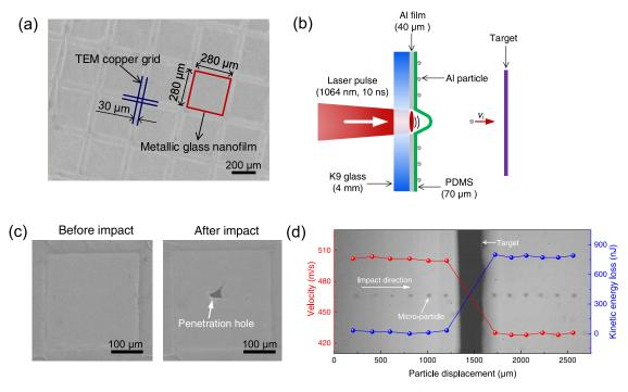
**Figure 1.** Laser-induced micro-particle impact testing (LIPIT) for the  $Ni_2Ta$  MG nanofilm. (a) Low-magnification SEM image showing the  $Ni_2Ta$  nanofilm supported by TEM copper grids. (b) Schematic diagram of the LIPIT platform. (c) SEM images of the  $Ni_2Ta$  nanofilm before and after perforation. (d) Multiframe snapshots show the velocity change and energy loss of the Al micro-particles during penetration at the speed of 500 m s<sup>-1</sup>.
