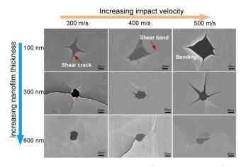
Figure 3. Postpenetration SEM images of the damage zone of the  $Ni_2Ta$  MG nanofilms with different thicknesses and impact velocities.
