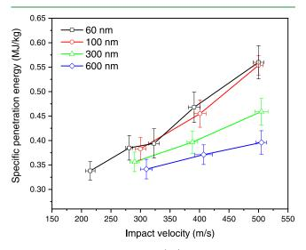
**Figure 2.** Specific penetration energy  $(E_p^*)$  of the Ni<sub>2</sub>Ta MG nanofilms with different thicknesses and impact velocities in micro-ballistic impact experiments.
