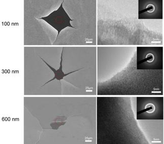
Figure 4. TEM images of fracture edges of the  $Ni_2Ta$  MG nanofilms with different thicknesses.
