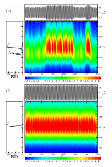
**Figure 8.** Frequency spectra of  $C_L$  in 3D wakes with  $L_Z = 4$  obtained through Morlet wavelet analysis at Reynolds numbers of (a) 240 and (b) 250.
