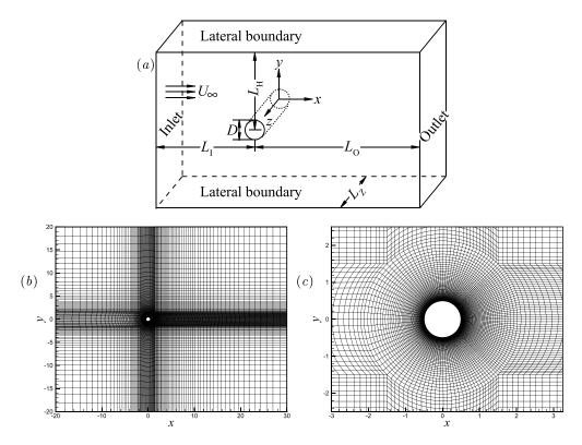
**Figure 1.** (a) Schematics of a flow past a straight cylinder with a circular cross-section, and computational domain in the (x, y) plane and mesh distributions in (b) the whole flow region and (c) near the cylinder with a closer view.
