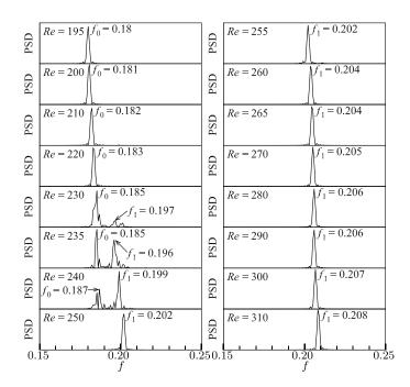
**Figure 6.** Frequency analysis of  $C_L(t)$  at different Reynolds numbers when  $L_Z = 4$ .
