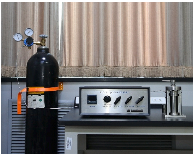
Fig. 4. Porosity measurement system.
