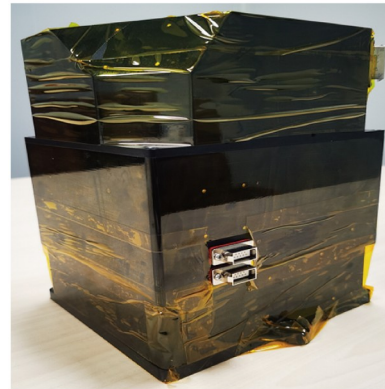
Figure 18 Picture of space curing verification platform for inorganic materials.
