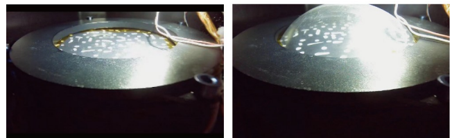
Figure 37 Image information of inorganic material cured and tested on-orbit (left: Pre-test; right: Post-test).
