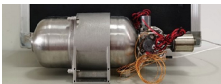
Figure 10 Picture of a high energy HAN-based unit liquid propulsion system.
