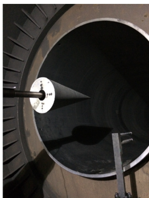
Fig. 13 Force test in JF-12 shock tunnel.
